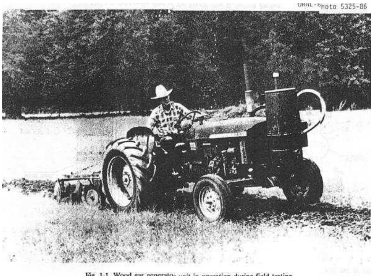
Fig. 1-1. Wood gas generator unit in operation during field testing.
