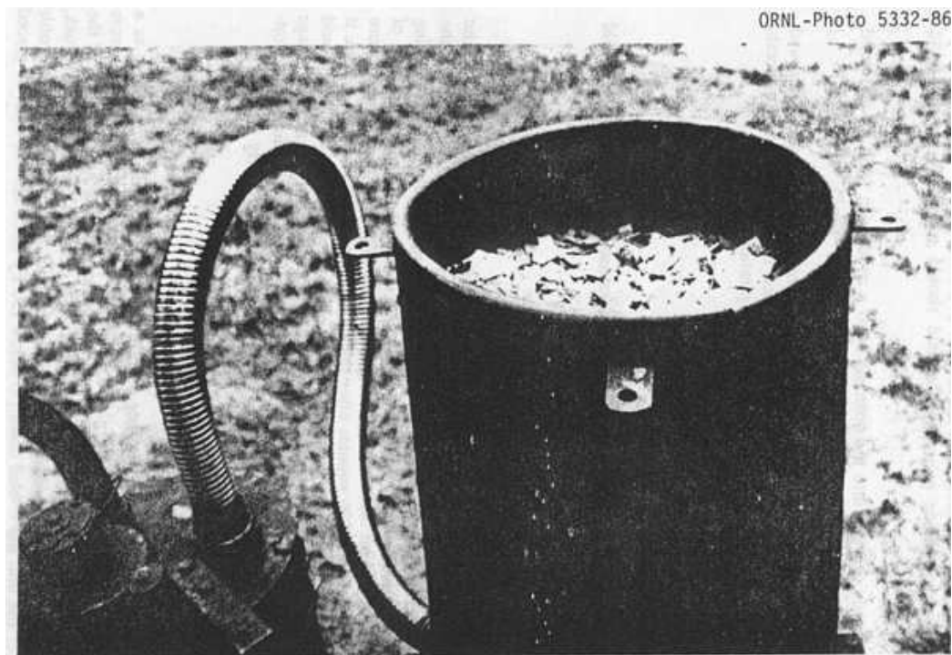
Fig. 3-1. Virtually all varieties of wood chips can be used for fuel. (Minimum size for this 6-in. firetube unit: 3/4 by 3/4 by 1/4 in.; maximum size: 2-in. cubes.)
